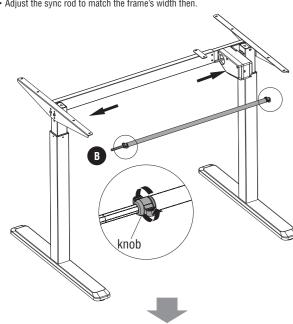
• Notice: Match the red line on the sync rod with the right side of left leg. Match the right side of the right knob of the sync rod with the red line on
