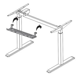
· Tighten all the screws on the hooks.
