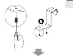
• Fix the hooks to the shelf with the previously removed screws.
